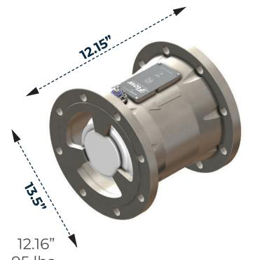
For best results install the Smart Valve downstream of water meter and backflow preventer (if present), but before any other equipment such as a pressure reducer or booster pump. Where possible it is recommended (but not critical) to have 10 diameters of pipe between the water meter and the valve. All flanged installations to use gaskets at each flange.
